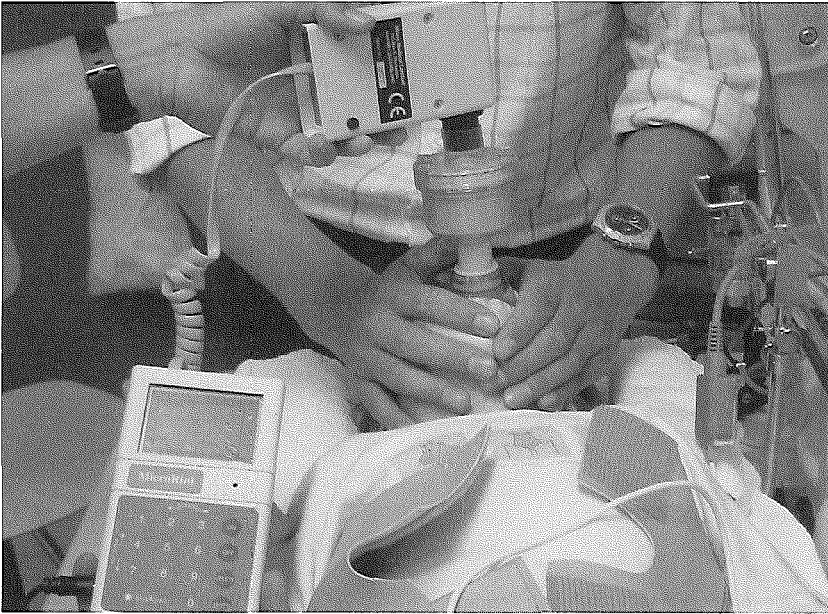
Figure 10. Resistance measurement using the interrupter technique ( R_{int} ) in a sedated infant.
