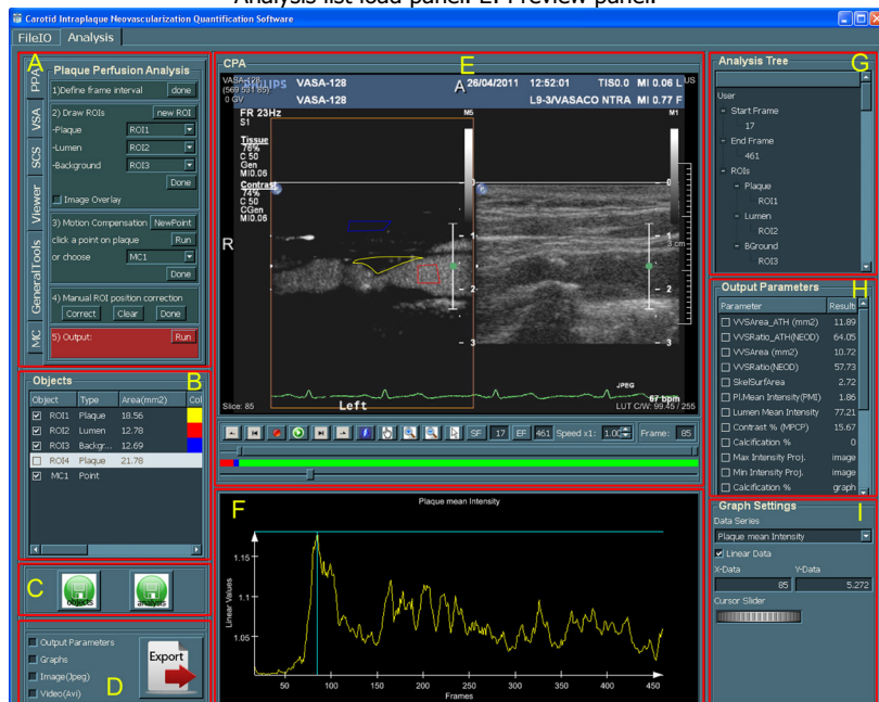
Figure 9: CINQS GUI - analysis part. A: analysis tools panel structured as a wizard. B: Object list panel. C: Saving object or analysis. D: Export results. E: Viewer panel. F: Graph panel. G: Analysis tree panel. H: Parameter output panel. I: Graph settings.
