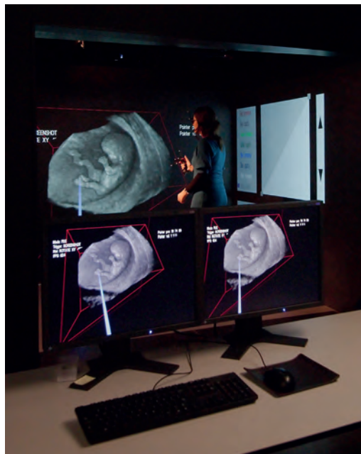
Figure 1: Image of the I-Space VR-system. Three-dimensional datasets are projected on the three walls and the floor of the room using eight projectors. An embryo of ten weeks and four days gestational age is visualized in the I-Space. The observer wears stereoscopic glasses and handles a wireless joystick to interact with the dataset.
