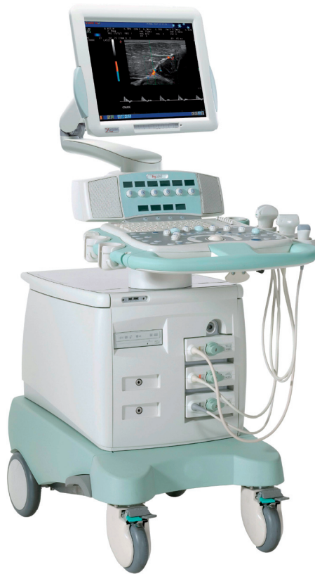
Figure 8: A modern US scanner. At the right hand side of the horizontal control panel there are 3 transducers. Directly underneath the screen is the vertical control panel. This modern scanner is mobile enough to move around.
