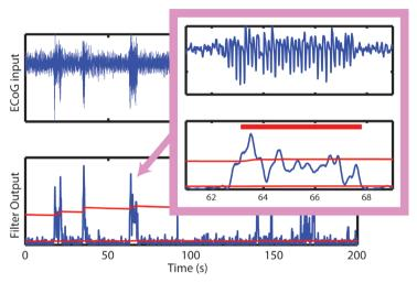
**Fig. 4.4** The input and output of the filter is shown with in the detail the response during the start of a seizure. The red lines correspond to the dual thresholds, while the thick red lines indicate when the output of the filter is enabled.
