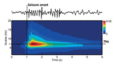
**Fig. 4.2** The average output of a continuous time complex Morlet wavelet filter over 1914 pre-recorded seizures. All seizures have a varying duration, but were aligned to have their onset at 1 s. The maximum output is obtained for the wavelet scale of 7Hz. A single seizure is plotted at the top of the figure for illustrative purposes.
