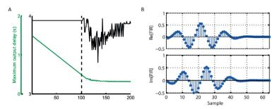
**Fig. 4.3 (A)** the trade-off between detection delay and wavelet precision as a function of the FIR truncation is shown. The green line is the detection delay and the black line shows the accuracy of the wavelet implementation. The black dotted line shows the chosen truncation setting at 101 samples for which the complex (i.e. real and imaginary) impulse response is shown in **(B)**.
