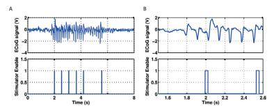
**Fig. 4.6** In vivo measurement results of the epilepsy detection system. After 4 GSWDs in the ECoG signal the detection is made and the stimulator is enabled, which subsequently suppresses the ictal activity. **(A)** the output during a full seizure is depicted, while in **(B)** the onset of the seizure is shown.
