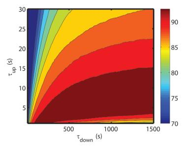
**Fig. 4.5** The Average Detection Rate (ADR) of the filter is given for various values of  $\tau_{up}$  and  $\tau_{down}$ .
