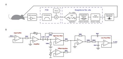
**Fig. 4.1 (A)** the closed-loop epilepsy detection system is depicted with the analog input filter (PCB) and the digital filter (Beaglebone) highlighted. **(B)** the implementation of the analog input filter is depicted that is used to make the recorded input signal suitable for digitization.
