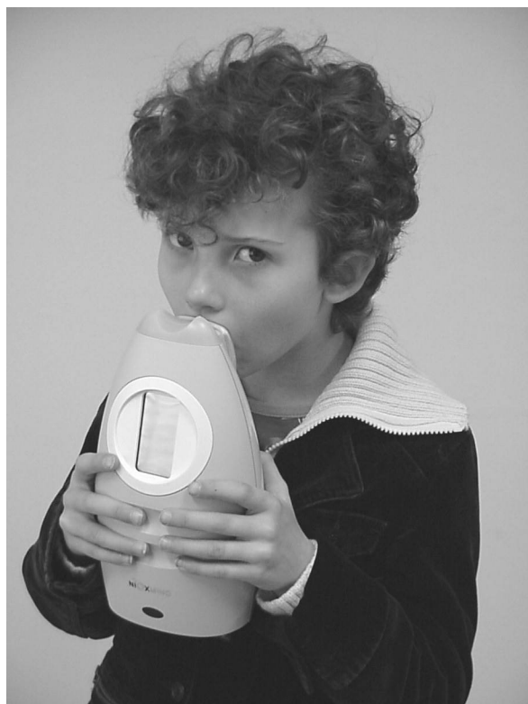
Figure 1.5 Six year old girl performing a single breath online manoeuvre with the NIOX MINO™, a portable NO-analyzer, that uses an electrochemical sensor. Deep inhalation through the mouthpiece provides NO-free air via an NO-scrubber. Next, exhalation for 10 sec with a constant flow of 50 ml/s is required. A visual and audible feedback system helps to maintain pressure within pre-set limits to ensure constant flow.
