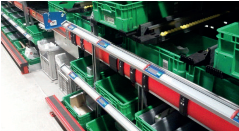
Figure 5. Picking station with automatic pick stock replenishment (Technische Unie, Alphen a/d Rijn)
