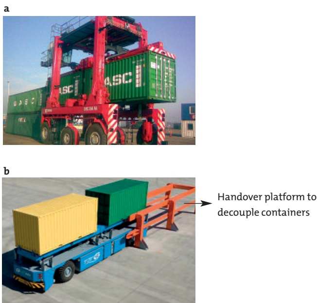
Figure 5. New internal transport vehicles: (a) Automated Lifting Vehicle, (b) L-AGV (Source: Gottwald Port Technology GmbH (2012))
