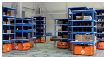
Fig. 3. KIVA system (top) and the shuttle system ADAPTO (bottom)
