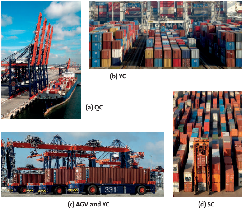
Figure 1. A top view of a container terminal and cargo handling equipment (Source: Europe Container Terminals (ECT), 2012)
