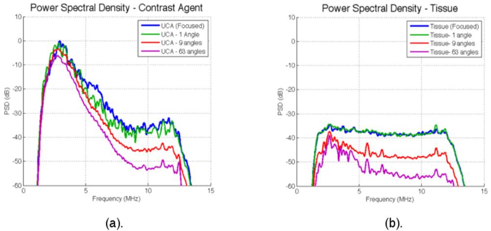
Figure 6.4 Power spectral densities of signals from UCA (left) and tissue (right) after AM processing, at 20 mm/s mean flow speed. Focused and Planewave  $N=1$  PSD are well-matched. Increasing  $N$  in Planewave reduces the broadband noise contribution at high frequencies.
