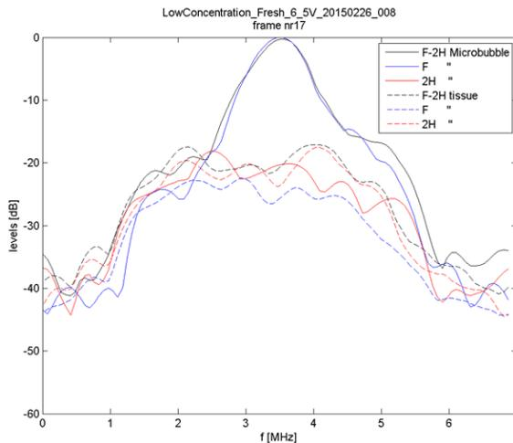
Figure 7:6 Spectra from the microbubble location and tissue location as obtained from the difference of two subsequent IQ-based images. For example, the " $F$  Microbubble" spectrum is obtained from the  $F_1 - F_2$  frames. The  $F-2H$  spectra are evaluated on the difference frame of two PM images, as depicted in Figure 4 (far right). The difference step further reduces residual tissue levels to below the noise floor.
