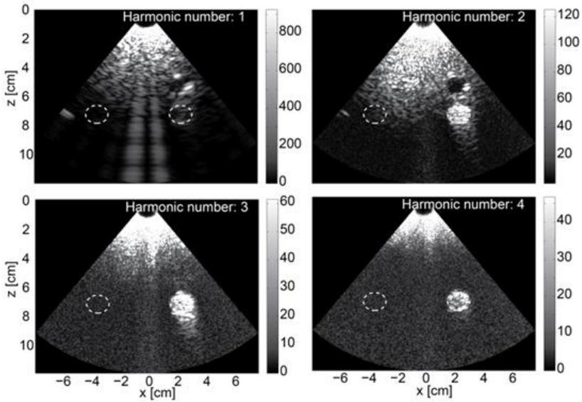
Figure 4:11 Images obtained from the experiment after spectral separation of the subsequent harmonics
