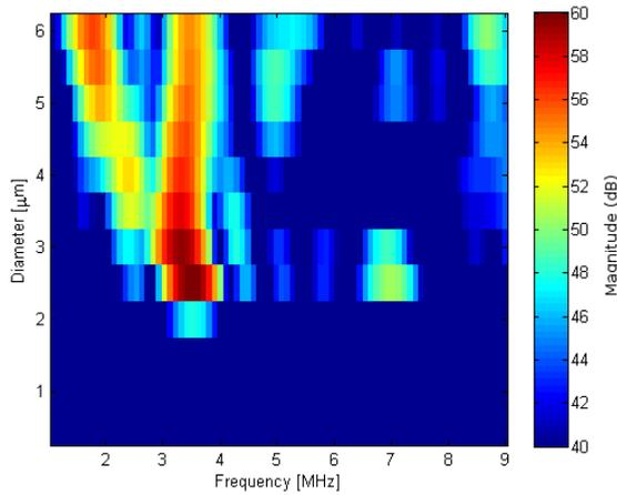
Figure 6.7 Simulation results for a single, isolated bubble, of parametric radius, after AM was applied. For this simulation, a full Marmottant model was used, with  $\kappa_s = 6 \times 10^{-9}$ ;  $\chi = 2.5 \text{ N/m}$ ,  $\sigma_0 = 0.5 \text{ N/m}$ ;  $\sigma_w = 0.036 \text{ N/m}$
