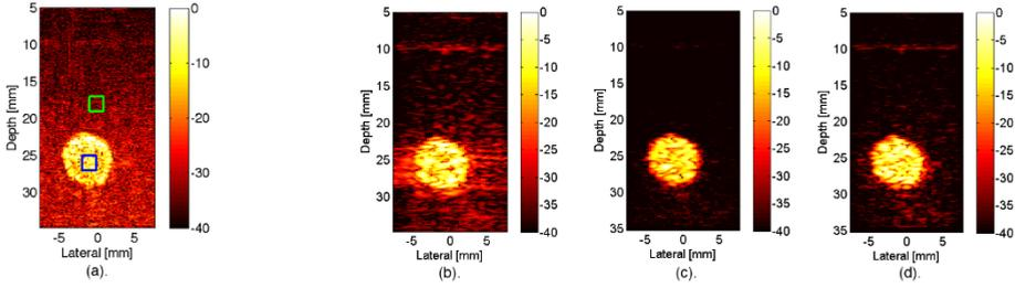
Figure 6.2 Left to right: Focused AM (a) ; Compounded Planewave AM with increasing number of angles ( $N = 1; 15; 63$ , respectively). Fig. (a) also shows the ROIs for evaluation of UCA (blue) and background (green) signal intensity.
