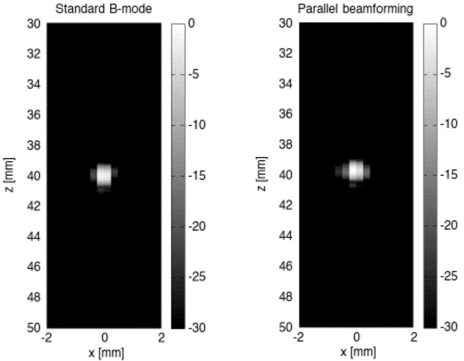
Figure 4.8 Standard B-mode and parallel beamformed second harmonic image, obtained with a single beam (beam 2) and three parallel beams, respectively. The pulse length is  $3 \mu\text{s}$ , the frequency separation  $f_s$  is 1 MHz and the cutoff frequency is 0.5 MHz. Intensity values are in dB.
