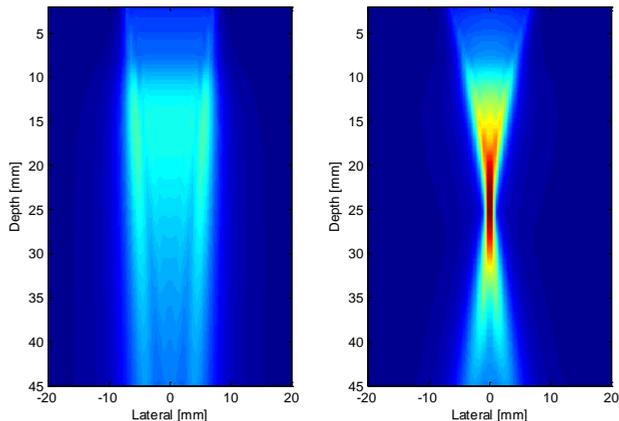
*Figure 8:2 Simulated pressure distribution. Left Plane wave, right focused beam. The peak pressure point in plane wave transmission (left) is located at 18mm, at the focus of a simulated acoustical lens that focuses the beam on the elevation-depth plane (not shown). For a simulation with 64 active elements, the peak pressure for plane wave is 4 times less intense than the focused case.*
