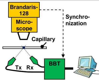
Figure 3:1 Schematic drawing of the setup. The Brandaris camera acts as master, triggering the BBT system to start US transmission and recording. Although the RX capability is not exploited in this work, this setup is suitable for acoustical recordings of single bubbles using separate TX and RX transducers.
