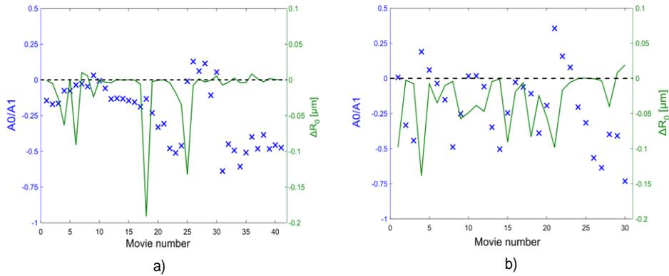
Figure 3:5  $A_0/A_1$  ratio versus record number (blue crosses) and changes in the resting radius ( $\Delta R_0$ ) versus record number (green solid line). A. (left) refers to the bubble recordings shown in Fig. 3 (single frequency). B. (right) refers to the bubble recordings shown in Fig. 4 (Step-FM). In both examples it can be noted that near a discrete radius decrease, the  $A_0/A_1$  ratio increases, eventually leading to a predominantly expansion-only behavior.
