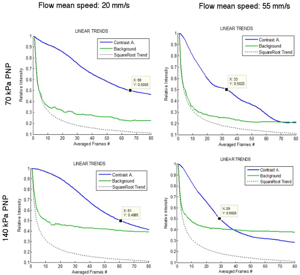
Figure 6:5 Relative intensity of UCA and background when multiple planewave ( $N=1$ ) frames are averaged. The number of averaged frames at which the contrast relative intensity is halved is highlighted. The 2x2 cartesian product set is shown here for two different  $P$
