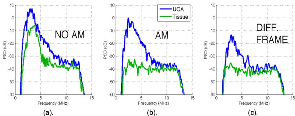
Figure 6:6 PSD of a single RF  $F$  frame (a), of an RF frame after AM processing ( $2H-F$ ) (b), and of the RF difference of two consecutive  $F$  frames ( $F_{i+1} - F_i$ ) (c). The 3.5 MHz peak after AM processing (b) is chosen as the 0 dB level for all of the three plots. In all cases, a strong UCA signal is visible, with the main peak being located at the fundamental frequency. The mean flow speed was 55 mm/s.
