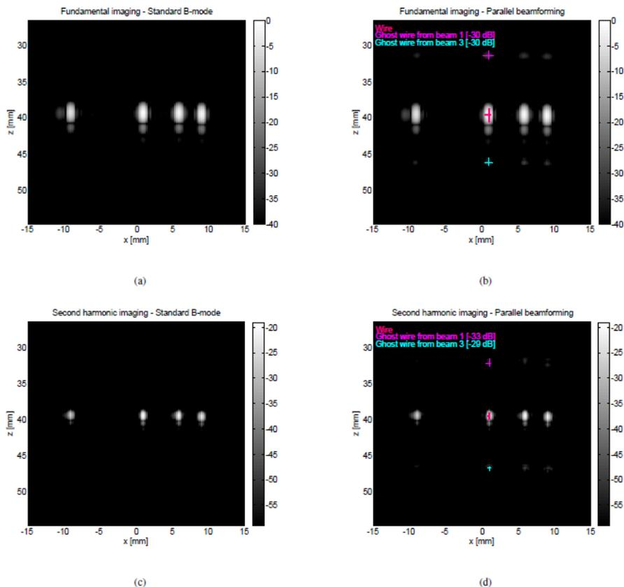
Figure 4.3 Standard B-mode and parallel beamformed, fundamental (a,b) and second harmonic (c,d) images as obtained with beam 2. The pulse length equals  $3 \mu\text{s}$ , the frequency separation  $f_s$  equals 1 MHz and the cutoff frequency equals 0.25 MHz in case of fundamental imaging and 0.5 MHz in case of second harmonic imaging
