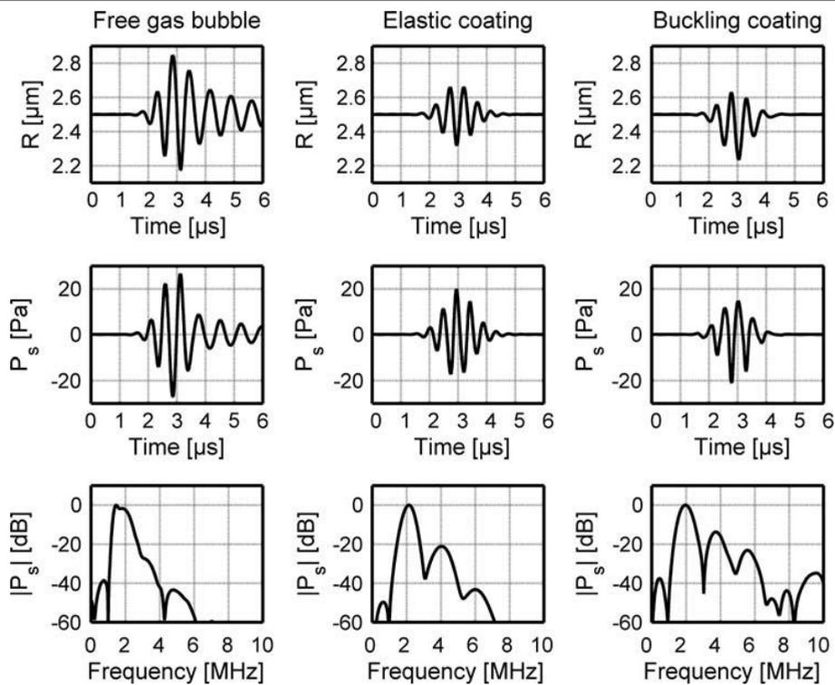
Figure 2:3 Vibration of a 2.5- $\mu\text{m}$  free bubble and coated bubble ( $\nu = 0.55 \text{ N/m}$  and  $j_s = 2.3 \times 10^8 \text{ kg/s}$ ) at 2 MHz in water. Top radial oscillation, Middle scattered pressure at 1 cm, Bottom frequency response of scattered pressure. {Source: Jong, N., M. Emmer, et al. (2009). "Ultrasonic characterization of ultrasound contrast agents." *Med Biol Eng Comput* 47(8): 861-873 }
