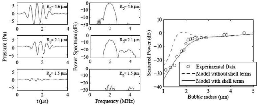
Figure 2:11 Measured responses of three single bubbles of three different sizes (4.6, 2.1 and 1.5  $\mu\text{m}$ ) excited with a driving pressure of 100 kPa. Left panel Measured pressure in Pa. Right Panel frequency response (reproduced with permission of JASA 2008)
