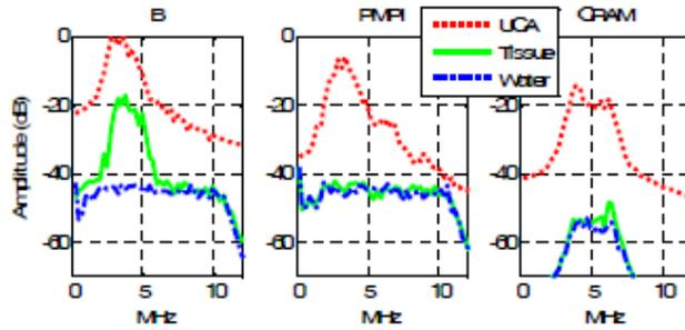
Figure 5.3: Average spectra computed over the 3 ROI for the contrast methods shown in figure 2, normalized to the absolute maximum amplitude. In these graph the transducer frequency compensation has been switched off.
