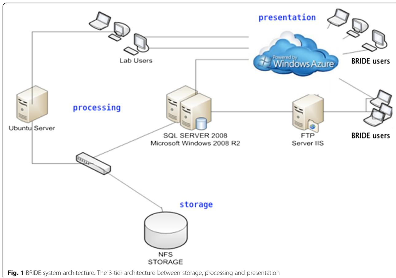
**Fig. 1** BRIDE system architecture. The 3-tier architecture between storage, processing and presentation
