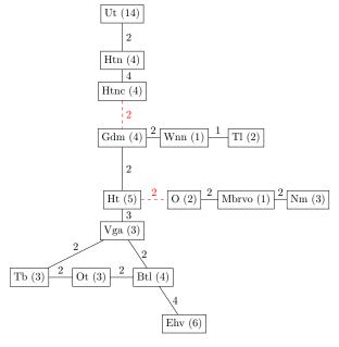
Figure 3: Graph of the railway network taken into account when rescheduling the timetable. Rectangles are the nodes and correspond to stations or important junctions. For each station, the number of tracks within the station is specified. Numbers at the edges indicate how many tracks connect two stations. The dashed edges represent the locations of the disruptions.
