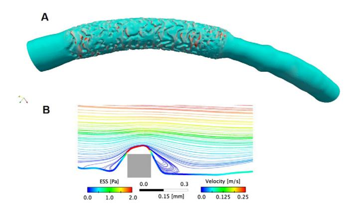
**Figure 5:** Recirculation zones(red) were quantified based on the ESS and the centerline direction (proximal  $\rightarrow$  distal). The red areas in the luminal surface are where the vectors of the ESS are pointing opposite (more than 90-degrees away from) the proximal-to-distal direction along the centerline (A). Rectangular cross-section induce recirculations upstream and downstream of the struts (B)
